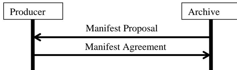
This sequence diagram differs from 5.2.1.1 in representing a ‘pull’ model where the archive informs the producer of the records that the archive is willing to take custody of. An example of this approach is where an organization retrieves records from a secondary storage supplier.
